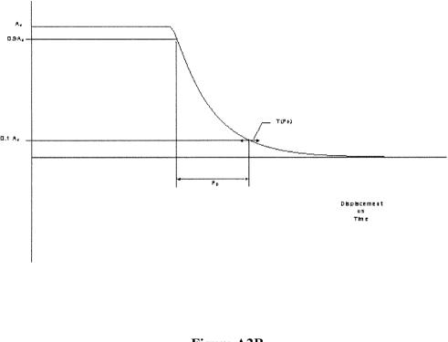
Figure A2B Critically and Overdamped Step Response
